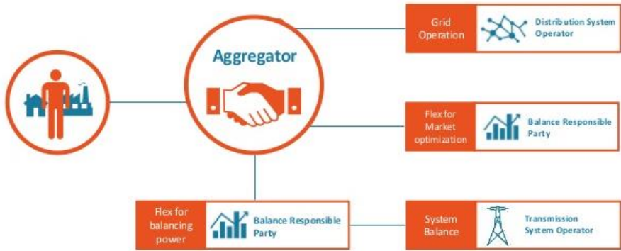
Figure 2: The role of the aggregator between the balancing resource owner and the market [10].
