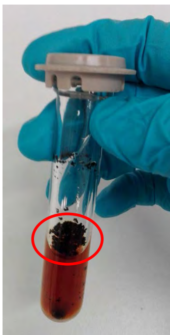
Fig. A5. Furfural and humin formation under auto-catalyzed conditions at 190 °C in 60 min employing 3 ml of birch hydrolysate.
