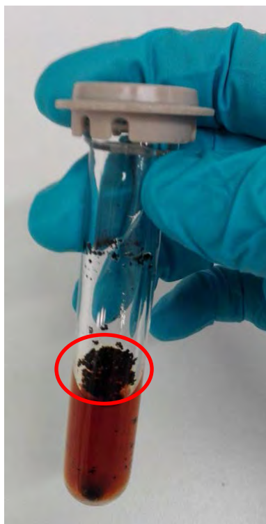
Figure 24. Humin formation under auto-catalysed dehydration of hydrolysate liquor at 190 °C in 60 min ( Paper IV ).
