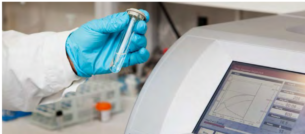
Figure 9. Valorisation of hemicelluloses using a microwave reactor (Monowave 300, Anton Paar GmbH, Graz, Austria) in papers I, II and IV.
