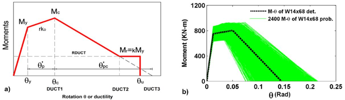
Figure 5. a) Modified IMK model: monotonic curve; b) an example of the modified IMK model used in the structural section (W14x68) of the probabilistic models.
