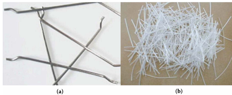
Figure 3. (a) Steel structural macrofibres; and (b) synthetic structural macrofibres.
