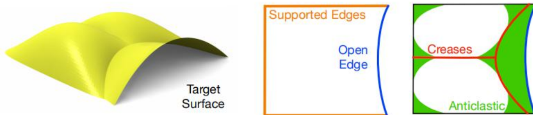
Fig. 9. The positions of the open edge (blue line) and the creases (red line) in the target surface [25]
