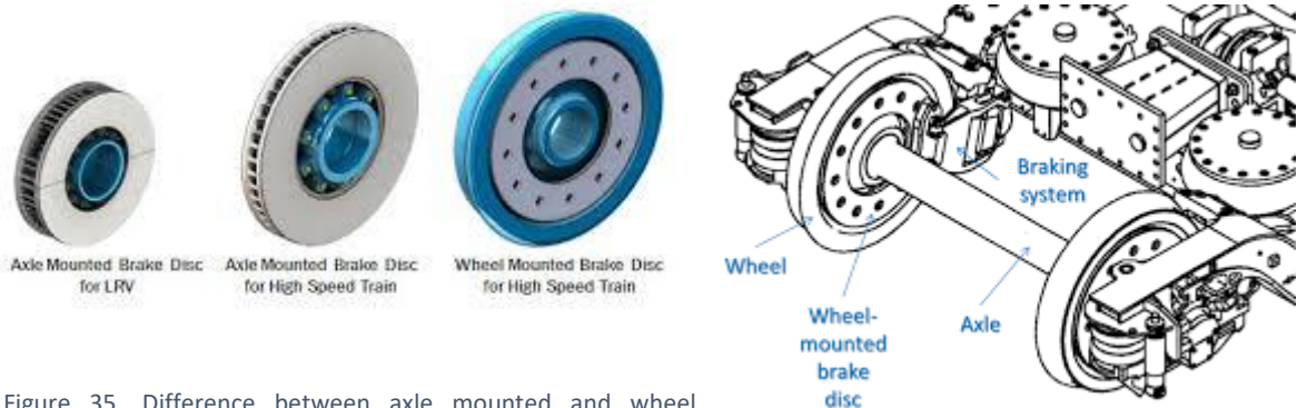
Figure 34. Setup of a wheel mounted disc brake [48].
