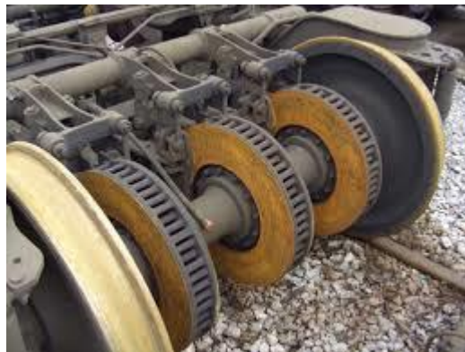
Figure 33. Axle mounted disc brakes on a high-speed train [20].
