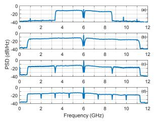
Fig. 6. Power Spectral Density of the received signal (with a received optical power of -25 dBm) for (a) 2.5 GBd full-band CAP, (b) 5 GBd full-band CAP, (c)  $2 \times 2.5$  GBd multiCAP, (d)  $4 \times 1.25$  GBd multiCAP.
