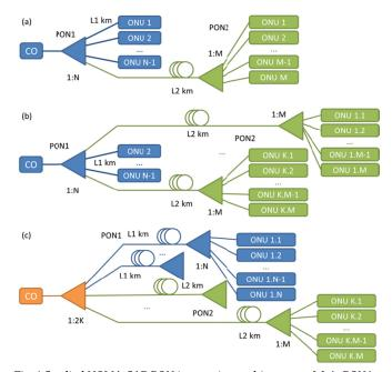
Fig. 4 Studied NOMA-CAP PON integration architectures: (a) 1×PON1 + 1×PON2; (b) 1×PON1+k×PON2, (c) k×PON1 + k×PON2, from [13].
