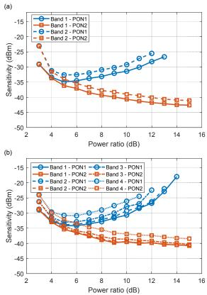
Fig. 8. Sensitivities at the 7% FEC limit for PON1 and PON2 users as a function of the power ratio and received power for two-band multiCAP (2×2.5 GBd) (a) and four-band multiCAP (4×1.25 GBd) (b).
