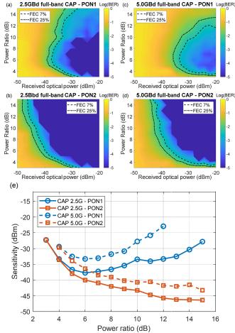
Fig. 7. BER and FEC limits for PON1 and PON2 users as a function of the power ratio and received power for 2.5 GBd (a-b), 5 GBd (c-d) full-band CAP and (e) sensitivities at the 7% FEC limit.
