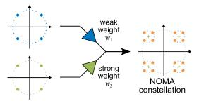
Fig. 3. Two users Non-Orthogonal Multiple Access constellation multiplexing, from [12].
