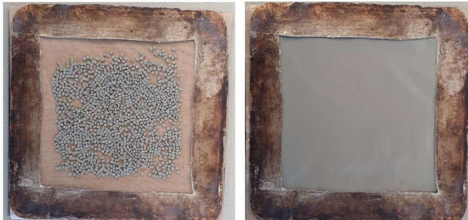
Figure 16. Steps of compression moulding. Before and after compression process.
