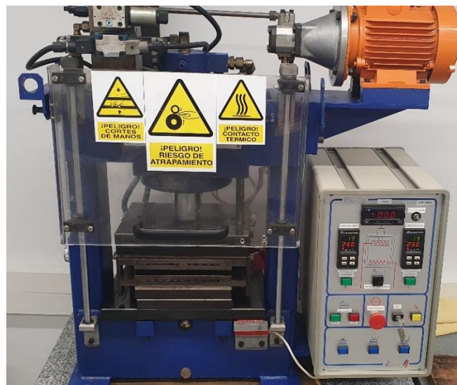
Figure 15. Compression moulding machine, model PL-15, IQAP-LAP, used in this work.
