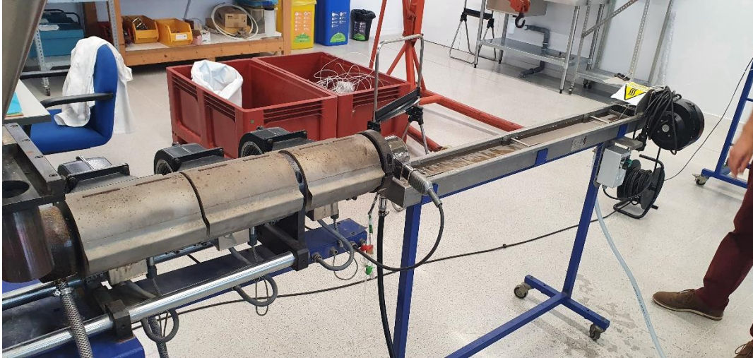
Figure 12. Extrusion setup for homogenising recycled PET flakes.
