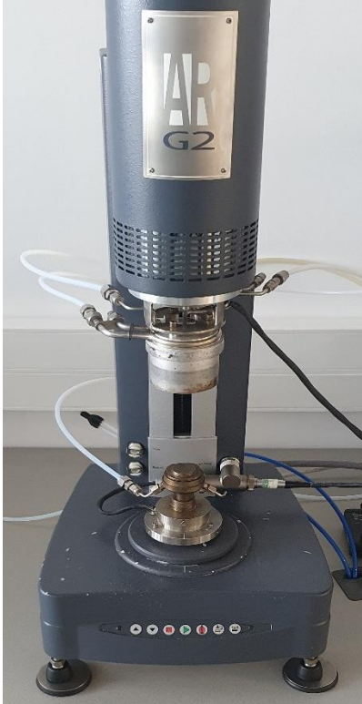
Figure 18. AR G2 rheometer on which rheological tests were performed.
