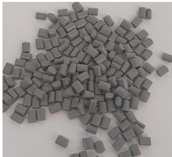
Figure 13. Visual appearance of pellets after extrusion
