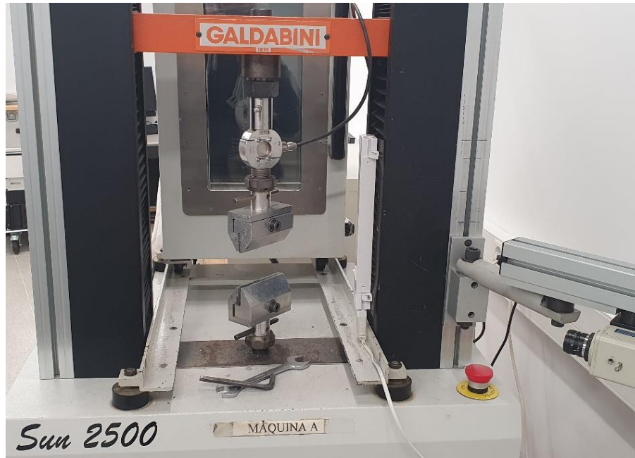
Figure 23. Galdabini Sun 2500 tensile testing machine. On the right is the camera for the video extensometer.
