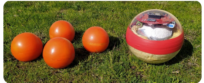
Fig. 3. At left, four WAVY Littoral drifters developed by MELOA consortium, at right, the ocean drifter prototype.
