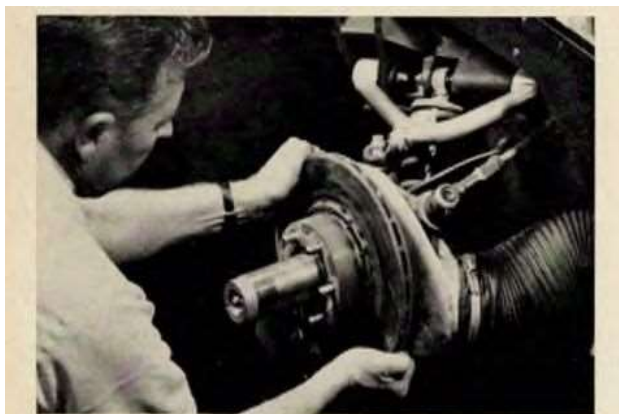
Phil Remington demonstrates the ease with which the brake discs are removed. Two bolts hold caliper in place, and wheel itself locates the disc's hat section axially.
