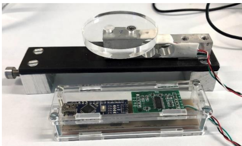
Figure 4.14 Force measuring module. [own source]
