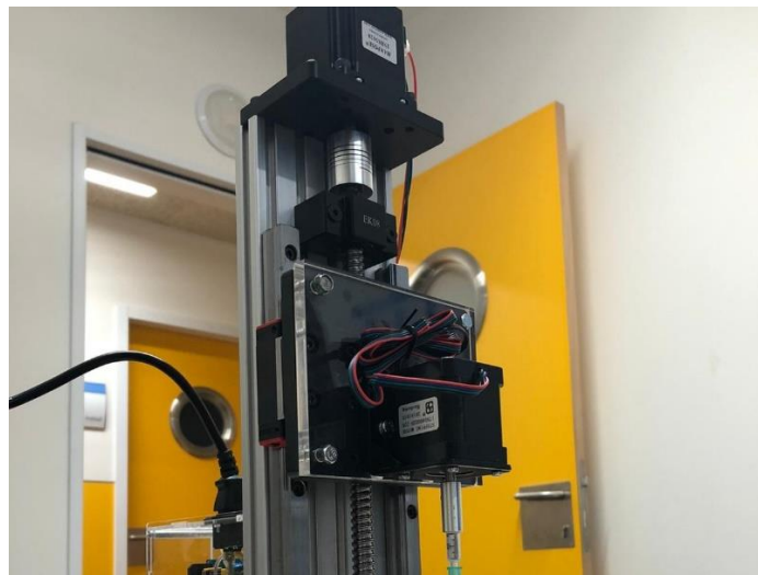
Figure 5.1 Linear actuator leadscrew and its needle support. [Own Source]
