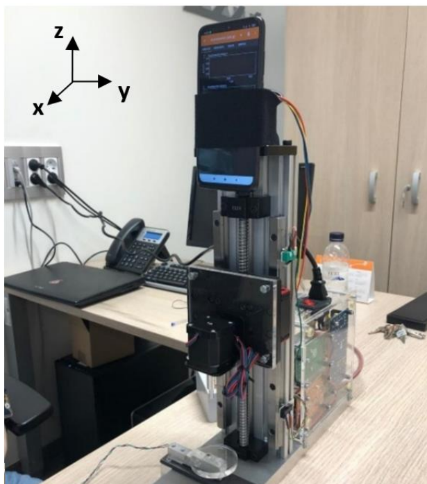
Figure 5.7 Setup to record vibration with the Mobil phone and the Phypox app. [Own Source]
