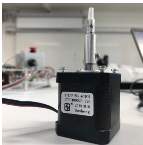
Figure 4.8 Stepper with the universal needle adapter. [Own Source]
