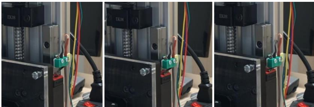
Figure 4.13 Moving plate interfering with the limit switch and consequently stopping the movement. [Own Source]
