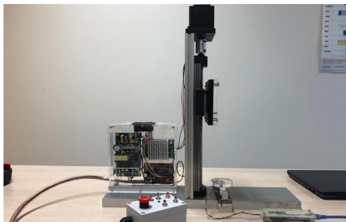
Figure 4.6 inverted T-shaped linear actuator structure.
