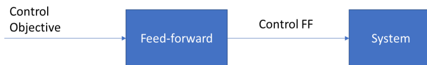
FIGURE 1.11: Feed-forward controller scheme.
