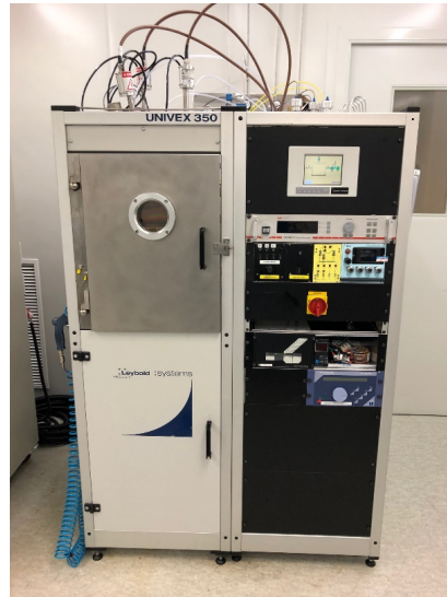
Figure 6: Leybold Systems UNIVEX 350 Sputtering machine from UPC clean room.
