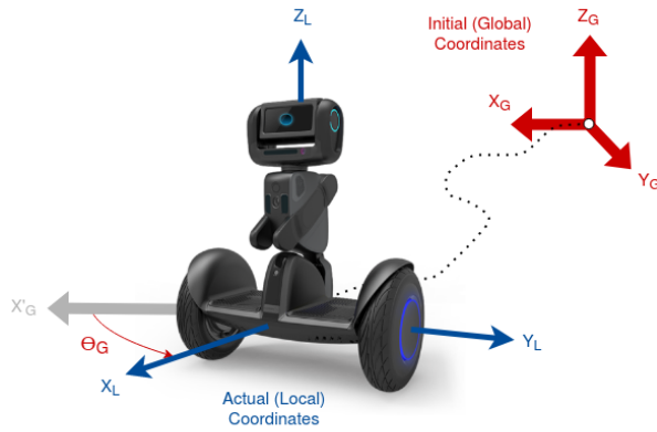
Figure 5: Loomo coordinate system. We use it in all the structure pillars. The global axis is represented in red, while the local one in blue. The heading angle ( \theta_G ) goes from global x -axis to local x -axis.
