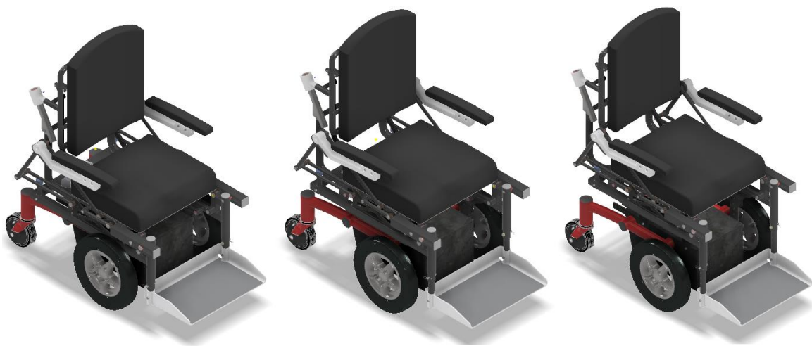
Figure 4-7 Isometric view of the final 3D model (Autodesk Inventor) with different adaptability settings in its initial position. (Left: Shortest; Middle: Medium; Right: Largest)
