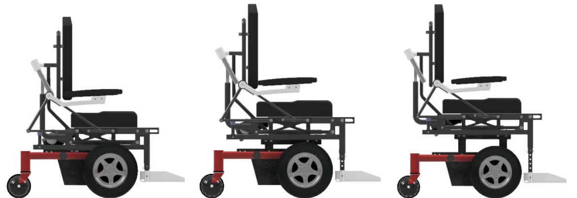
Figure 4-9 Side view of the final 3D model (Autodesk Inventor) with different adaptability settings in its initial position. (Left: Shortest; Middle: Medium; Right: Largest)
