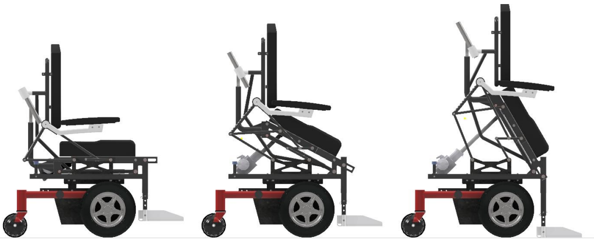
Figure 4-6 Lateral view of the final 3D model (Autodesk Inventor) with its transition from initial to end position.
