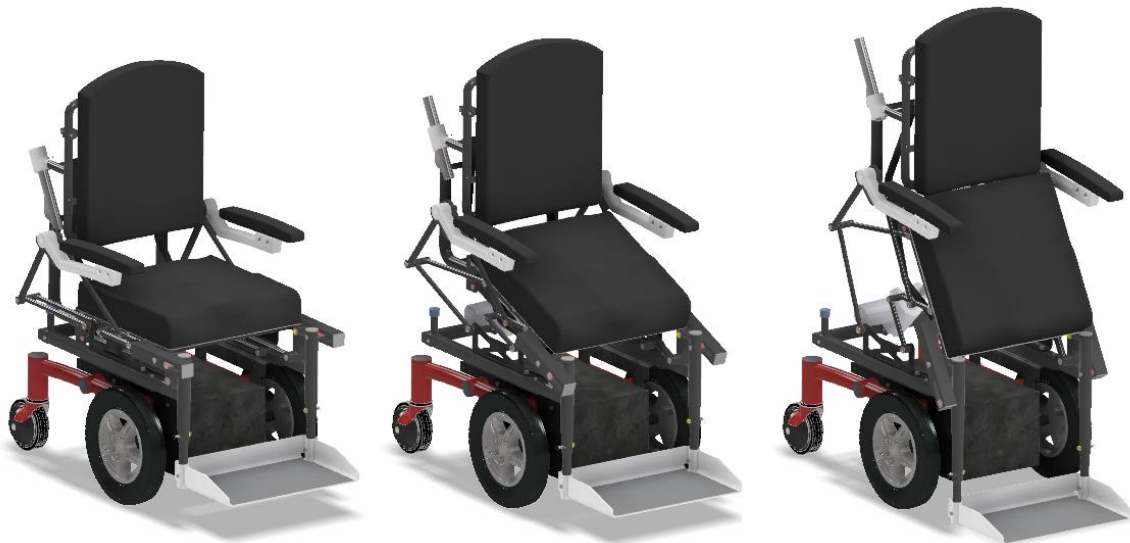
Figure 4-5 Isometric view of the final 3D model (Autodesk Inventor) with its transition from initial to end position.
