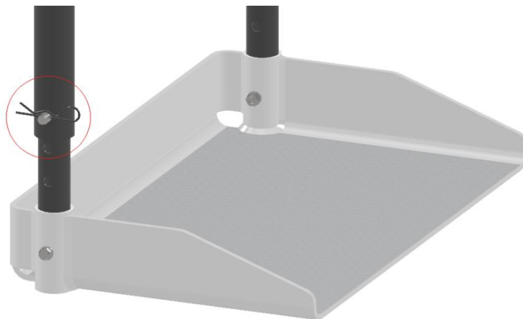
Figure 4-33 Hitch Pin and R-Clip system of footrest telescopic system.
