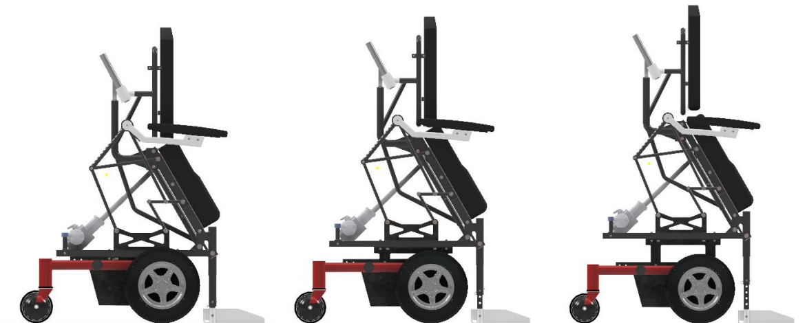
Figure 4-10 Side view of the final 3D model (Autodesk Inventor) with different adaptability settings in its end position. (Left: Shortest; Middle: Medium; Right: Largest).
