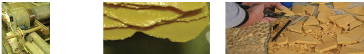
Figure 2. Left: Murano Smalti glass forming process by lamination until flat piastras are obtained. Center: glass piastras shown on Side 1. Right: manual cutting process (source: authors).
