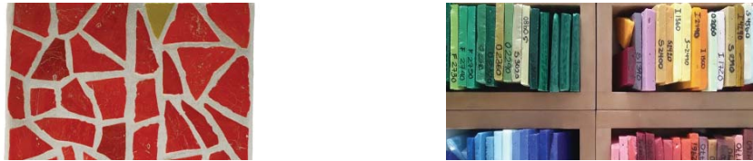
Figure 1. Left: test piece for trencadís coating tests made with smalti Murano glass tiles. Right: referenced glass samples analyzed in this study(source: authors).
