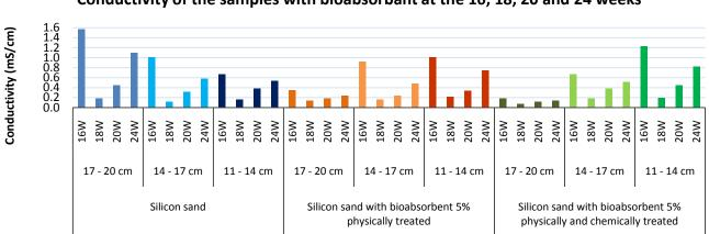
Conductivity of the samples with bioabsorbant at the 16, 18, 20 and 24 weeks
