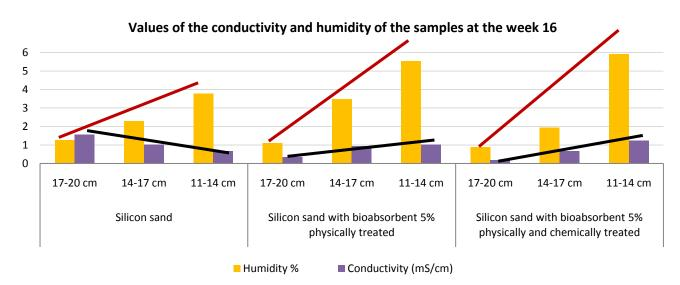
FIGURE 5: Values of the conductivity and humidity of the samples at the week 16
