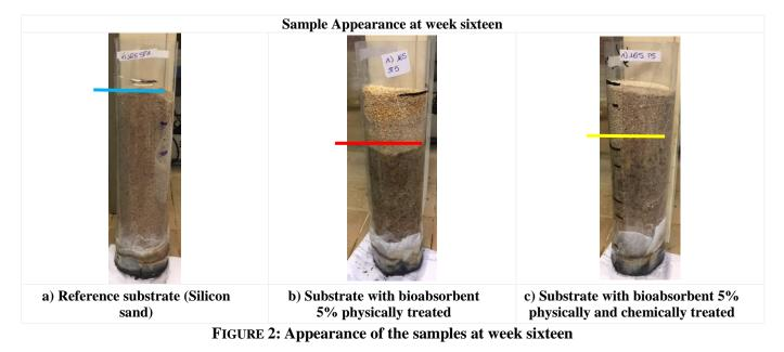
The rise of the water corroborated the interaction of the seawater and the bioabsorbent. The parameters measured were the pH, humidity and conductivity. The substrate was inside a PVC tube divided into four sections (Figure 3): the first one between the base of the tube and 11 cm, the second section between 11 - 14 cm, the third between 14 - 17 cm, and the last one on the surface of the tube 17 - 20 cm.
