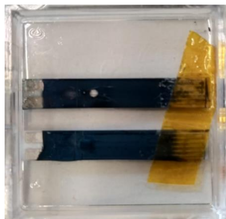
Figure 9: Both sensors mounted on a board with the WO 3 layer
