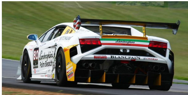
FIGURE 1.8: Racing car with spoiler and diffuser [6]
