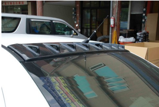
FIGURE 1.12: Strip of VGs on a racing car [8]
