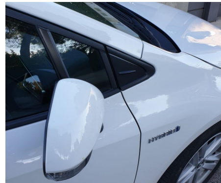
FIGURE 1.13: VG located next to the mirror
