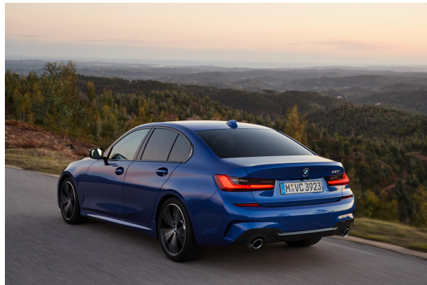
FIGURE 1.9: Vortex generator (Shark fin shape) on top of the BMW 3 series [5]
