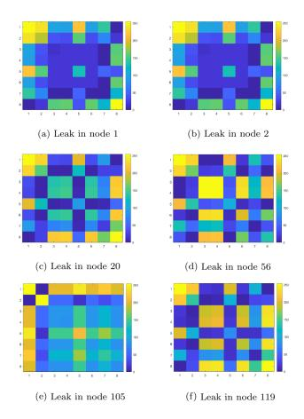
Fig. 5. GAF images associated to different leaks
