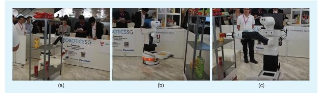
Figure 5. The Robotics.SG demonstration. TIAGO (a) retrieves a bin with returned items, (b) navigates a store by using a prerecorded map, and (c) places an item on the required shelf.
