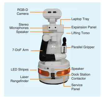
Figure 2. The TIAGo wheeled manipulation platform.
