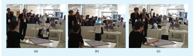
Figure 4. The TAMS demonstration. (a) A user points at a menu to order a drink. (b) TIAGo moves to a bar to retrieve the liquor. (c) The robot pours the (real) liquor into a glass.
