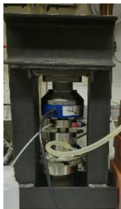
Figure 3.15. Load cell that measures the swelling pressure
