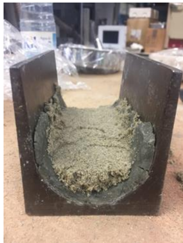
Figure 4.3. First trial test at 65% of water content MX-80 bentonite
