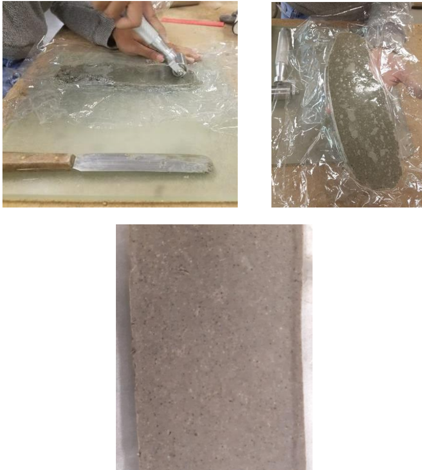
Figure 4.4. Second trial test at 70% of water content MX-80 bentonite
