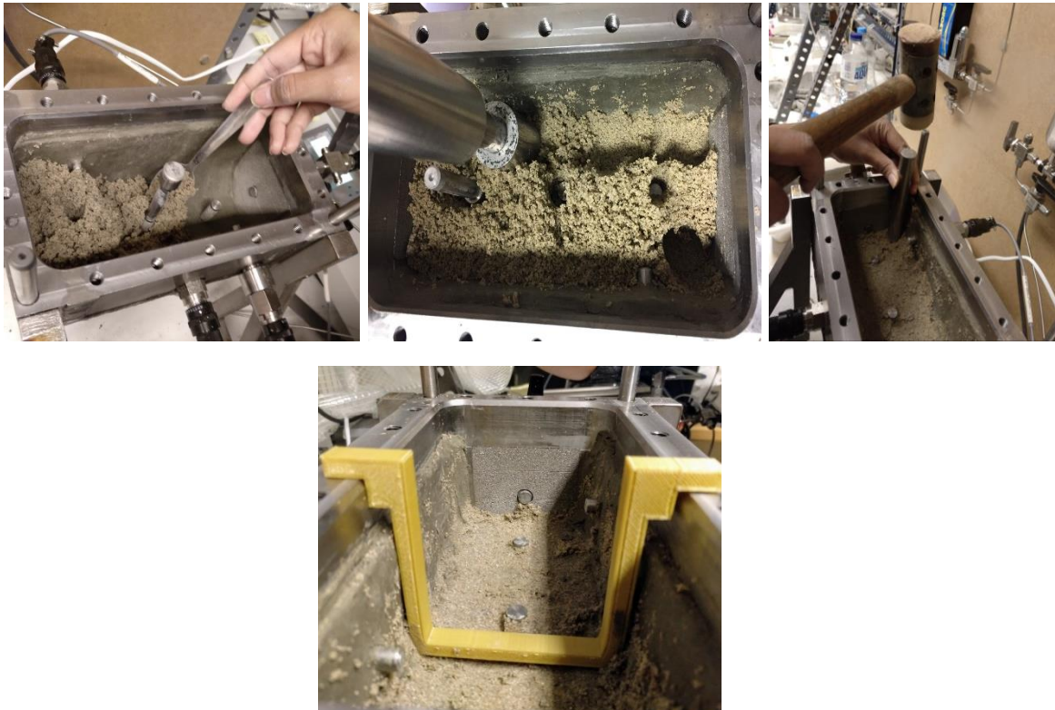
Figure 3.11. Sand/bentonite placed inside MU-B cell.
