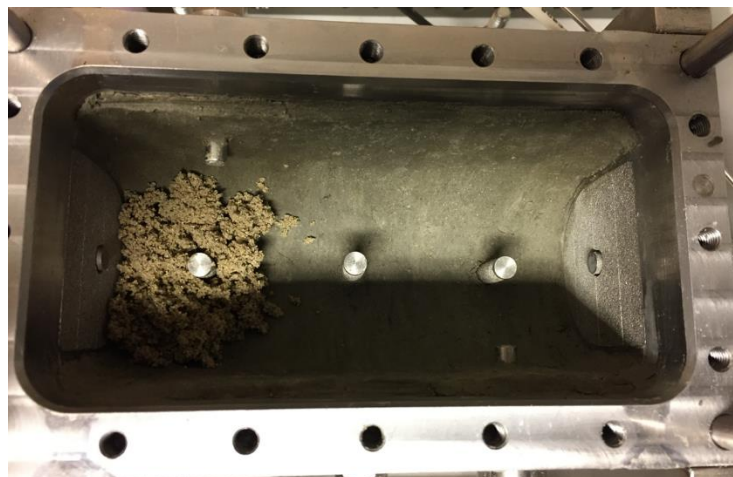
Figure 4.7. Third trial test with MX-80 bentonite employed in MU-B equipment
