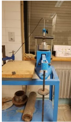
Figure 3.13. Conventional oedometer with load arm test for sand/bentonite (80/20)
