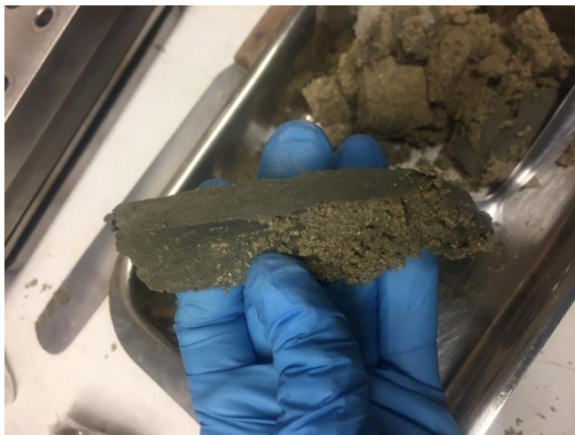
Figure 4.6. Extraction of MX-80 bentonite (right). Location of the samples extracted (left)
