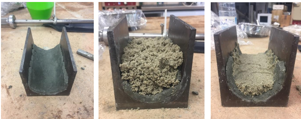
Figure 3.5. Compaction procedure in a prototype mould with MX-80 bentonite and sand/bentonite mixture, first test
