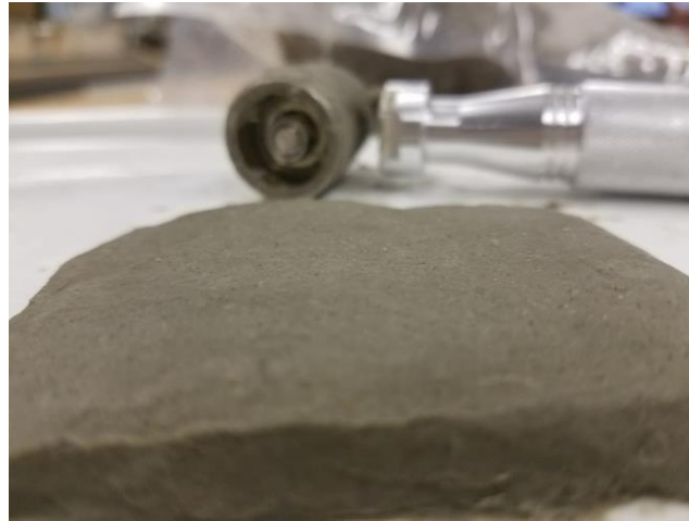
Figure 3.6. MX-80 bentonite with water content higher than the plastic limit, second test
