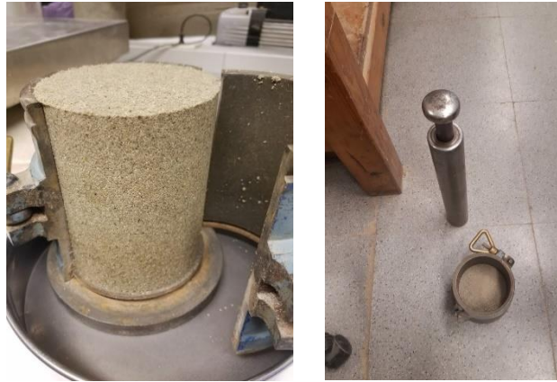
Figure 3.2. Standard proctor test to sand/bentonite (80/20)
