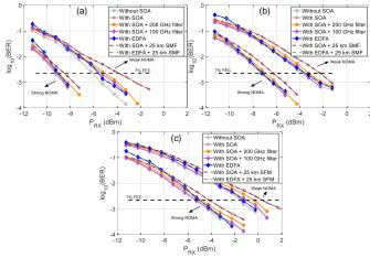
Fig. 2. BER vs. received power  $(P_{RX})$  for the strong and weak NOMA levels when the optical signal is amplified by SOA/EDFA and optionally filtered with 0 km and 25 km of SMF for: (a) 50 Gb/s, (b) 70 Gb/s and (c) 90 Gb/s.
