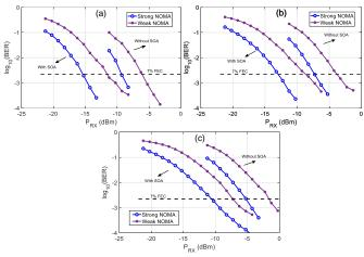
Fig. 3. BER vs. received power ( $P_{RX}$ ) comparison when the NOMA-CAP signal is pre-amplified by a SOA at the receiver and not with 25 km SMF for: (a) 50 Gb/s, (b) 70 Gb/s and (c) 90 Gb/s.
