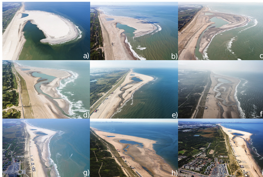
Figure 1. Aerial pictures of the first concentrated mega-nourishment (ZM, The Netherlands), showing its morphological evolution in the initial six years. Pictures were taken in: (a) July 2011 (shortly after construction); (b) October 2011; (c) January 2012; (d) October 2012; (e) October 2013; (f) September 2014; (g) May 2015; (h) August 2016; and (i) July 2017. Courtesy: Rijkswaterstaat, Joop van der Hout.
