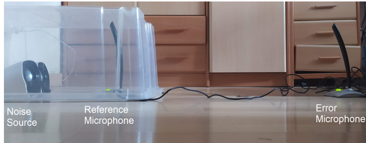
Figure 3.2: Audio reading system layout
