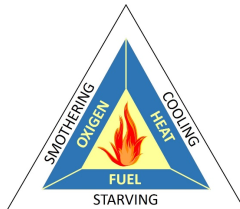
Suppression mechanisms within the fire triangle
