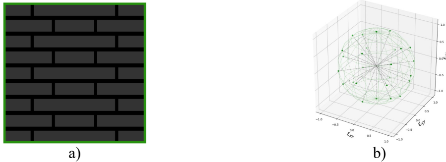
Figure 3: Virtual laboratory: a) Micro model of the representative volume element showing the brick units, the mortar joints and the boundary; b) generated strain database for the boundary displacement application
