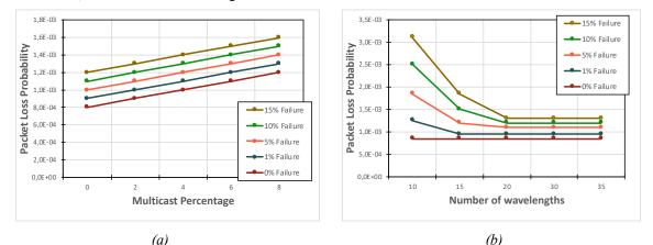
Failure 3. Packet loss probability as a function of failure probability: (a) multicast percentage and (b) WDM
