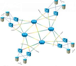
Figure 1. Proposed hybrid data centre network architecture
