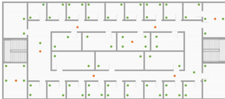
Figure 7: Sensor and gateway locations chosen by the model for the final optimized deployment.
