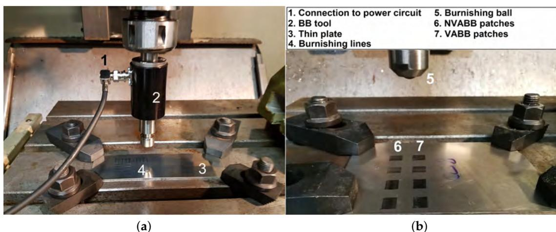
**Figure 1.** (a) Experimental setup of the ultrasonic vibration-assisted ball burnishing (UVABB) experiment. (b) Eight patches performed on the plate with a 10 wt.% of pre-existing martensite during phase 2.
