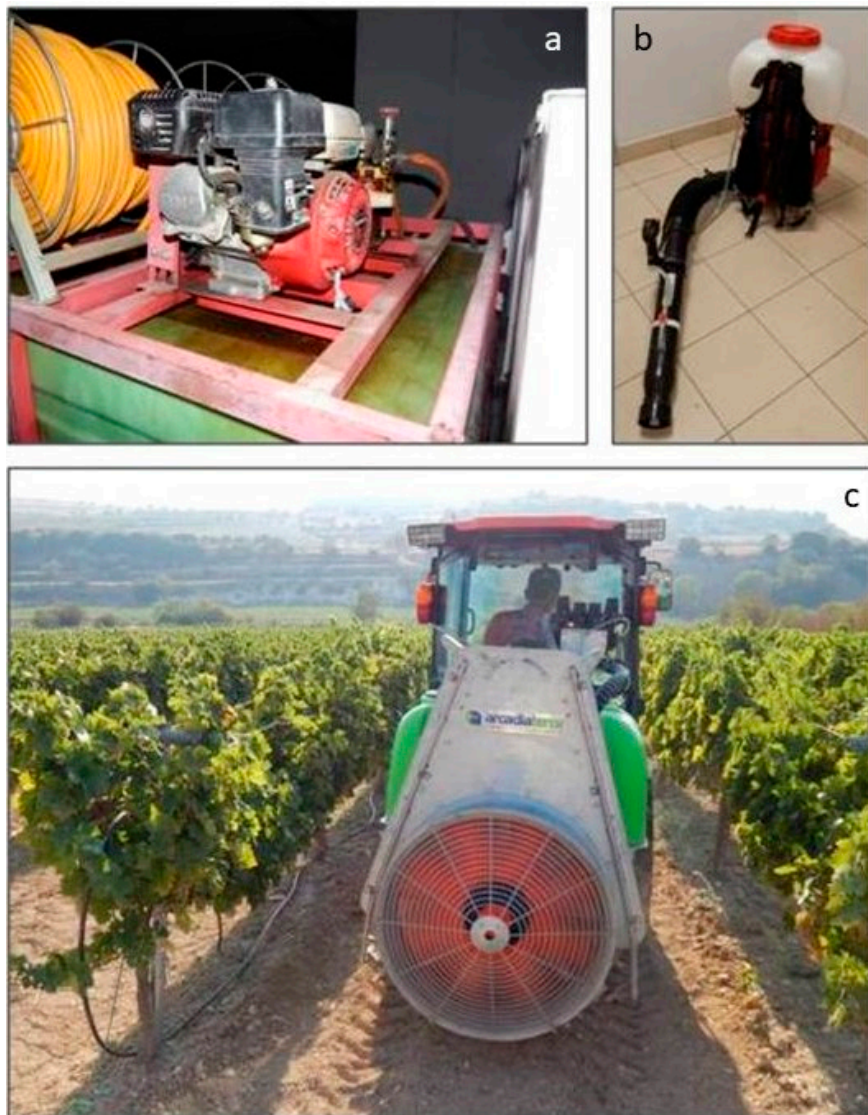
Figure 1. Sprayers tested: (a) HVS with a spray gun (b) LVS (Motorized knapsack sprayer) (c) OS (Axial fan orchard sprayer).
