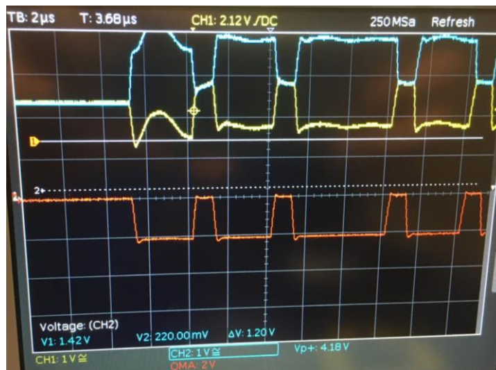
Figure 4.20: CAN sequence being transmitted
