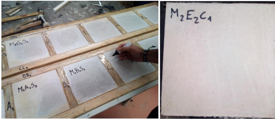
Figure 2. Manufacturing of specimens and traceability labels
