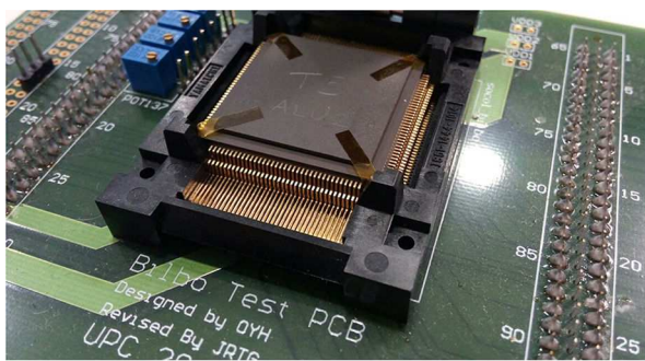
Fig. 11 Detail of the 144 pads encapsulated version of the fabricated IC mounted on the socket and soldered to the test printed circuit board
