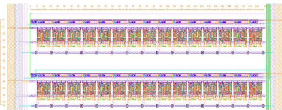
Fig. 8 Layout of the integrated signature generator subsystem (both channels), where the array of comparators can be appreciated as well the active voltage divider and the shift register structure. The integrated signature generator subsystem is 170\ \mu\text{m} wide and 62\ \mu\text{m} high ( 10,540\ \mu\text{m}^2 ) and has been designed and fabricated in an industrial 65\ \text{nm} STMicroelectronics bulk CMOS technology
