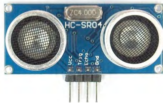
Figure 2. Schematic of an Ultrasonic ranging module HC-SR04.
