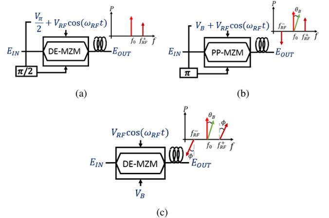
Fig. 5. Sketch of the typical options for external RF modulation at optical frequencies (a) DE-MZM configured for SSB modulation (b) Conventional push-pull MZM, and (c) DE-MZM for CD RF-amplitude free band control using the bias voltage.
