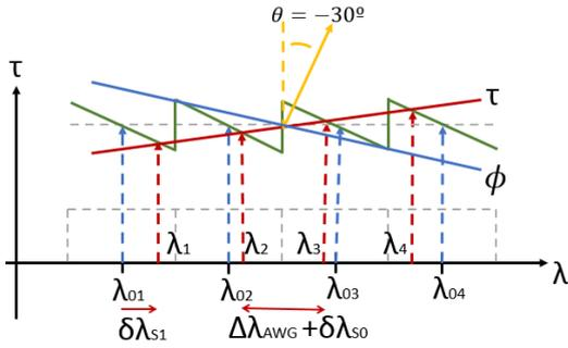
Fig. 4. Relative delays and beam direction for MW tuning.
