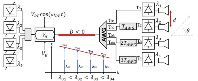
Fig. 1. Setup of OTTDN with DE-MZM.
