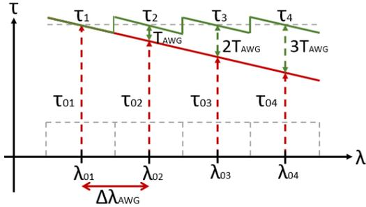
Fig. 2. Group delay distribution against wavelength at the PAAEs before (red) and after (green) compensating delays and relative PAAE channel spacing.
