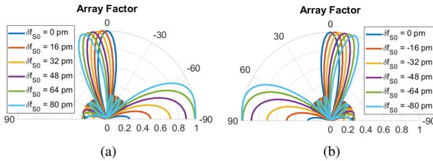
Fig. 6. Array Factor diagram for a relative progressive wavelength shift  $\delta\lambda_0 > 0$  (a) and  $\delta\lambda_0 < 0$  (b).
