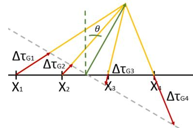
Fig. 3. Geometrical delays for each PAA element and beam direction  $\theta$ .
