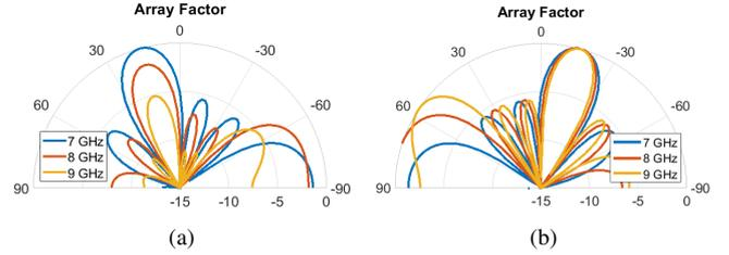
Fig. 7. Array Factor diagrams for  $\theta_B = \pi/2$  (a) and  $\theta_B = 1.35\pi$  (b).
