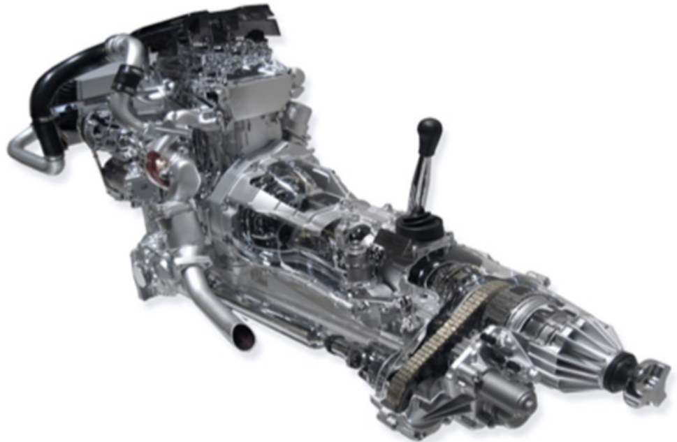
Figure 1 Nissan Pathfinder Engine. Characteristics: (i) 747 parts and 330 references (ii) 378 elemental assembly tasks grouped into 140 production line tasks.
