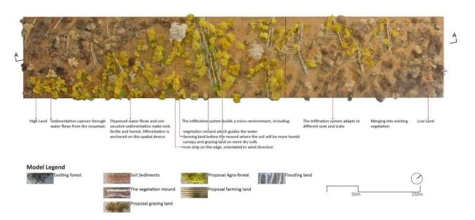
Fig. 04 The principle of cut and fill creating infiltration dams. They allow the water to infiltrate and slow down, divert and spread out over the territory as shown in the 1/500 model on the bottom. By irrigating the territory, deforested lands regain their vegetation and some agricultural practices can exist. Source:Project by Xiao Xinyu. (Xiao, 2018, p. 60)
