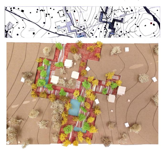
Fig. 09 On top the extraction design: the orthogonal logic is used for excavation, while following the lower part of the topography where water will accumulate. Below a zoom on the 1/500 model of brick oasis creek that is the result of a systemic extraction and inhabitation of the brick landscape. Project by Nathan De Feyter. Source:Nathan De Feyter.
