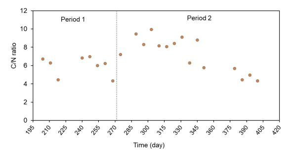
**Figure 7.** C/N ratio of the anaerobic digester influent (pretreated microalgal biomass) over the experimental periods 1 (HRT of 20 days) and 2 (HRT of 32 days).
