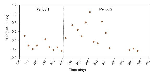
**Figure 5.** Organic loading rate in the anaerobic digester over the experimental periods 1 (HRT of 20 days) and 2 (HRT of 32 days).
