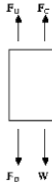
Figure 3.1 Summation of the forces acting on the tower at the geostationary height. Source: [6].
