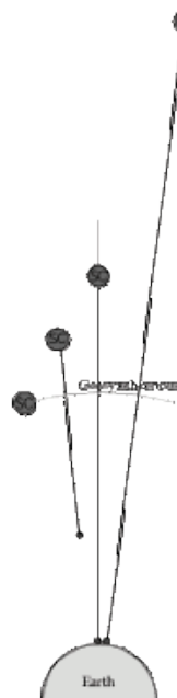
Figure 4.2 Deployment of the initial cable. The cable will be maintained at its geosynchronous orbit and the lower end of the cable will descend. Source: [1].
