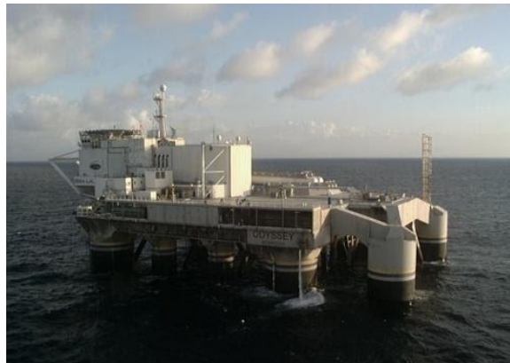
Figure 4.13 LP Odyssey, mobile spacecraft launch platform refurbished from an oil platform. Source: [22]
