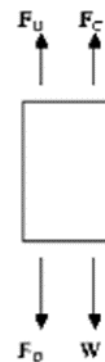
Figure 2.1 Summation of the forces acting on the tower at the geostationary height. Source: [3].
