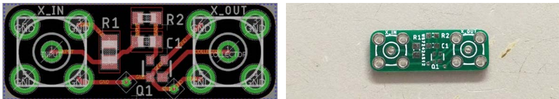
Figure 4.3: EAGLE schematic and photo of the PCB.
