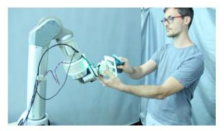
Fig. 1: Industrial scenario considered in this task. The operator can polish, grab the object or move the robot actuating over the shared object. Samples from the force sensor are used to classify user intentions, which change the robot behavior adaptively.
