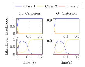
Fig. 3: Identifying user intentions. Network output: likelihood of the three possible intentions across time. In the window-based approach  $(O_w)$  the action is decided at fixed positions  $t_i$  depicted in the x-axis with discontinuous lines. In the confidence based approach  $(O_c)$ , the intention is decided when the likelihood of one action surpasses a certain threshold. In this example the threshold  $th_c$  has been set to 0.9.
