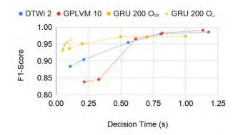
Fig. 7: RNN results with  $O_C$  confidence based decision.  $O_c$  confidence based criterion (GRU 200 confidence) reduce the mean inference time of getting a decision while increasing the F1-measure compared to  $O_w$  (GRU 200 window).
