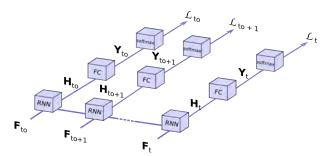
Fig. 2: Network's architecture. The network is displayed for multiple sensor measurements  $F_i$ . At each time instant the force sensor signals  $F_i$  are fed to the RNN, which updates the hidden states  $H_i$ . The fully connected layer (FC) uses  $H_i$  to obtain the user's intentions  $Y_i$ . User's intentions are converted to likelihoods  $\mathcal{L}_{t_i}$  with a softmax layer.
