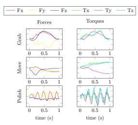
Fig. 4: Force/torque sensor data. The used dataset provides 6 signals: 3 forces and 3 torques axes. Each sequence is annotated with one of the three possible intentions of the user: grab, move or polish the object.
