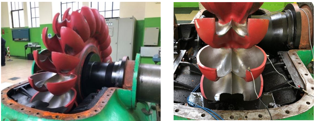
Figure 15. Left, runner 1-B attached to the machine and left, accelerometers placed on one bucket
