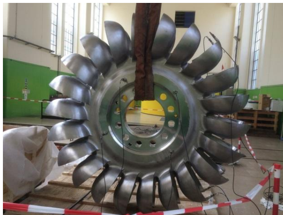
Figure 9. Accelerometers disposition on the hanged runner
