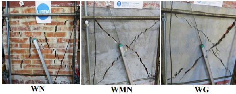
Figure 2. Specimen failures: WN, WNM, and WG
