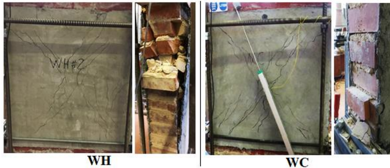
Figure 3. Specimen failures: WH and WC
