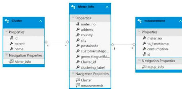
Fig. 3. Data model for the time-series measurements.
