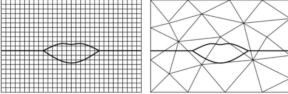
**Figure 3:** Two-grid method (2D sketch). The advection problems are solved on a structured grid of small cubic cells of typical size  $h_{cells}$  (left), and the diffusion problems are solved on an unstructured finite element mesh of typical size  $h_{fe}$  (right).
