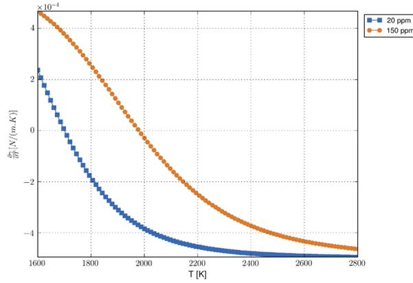
**Figure 4:** Surface tension derivative  $\gamma'(T)$  as a function of temperature.
