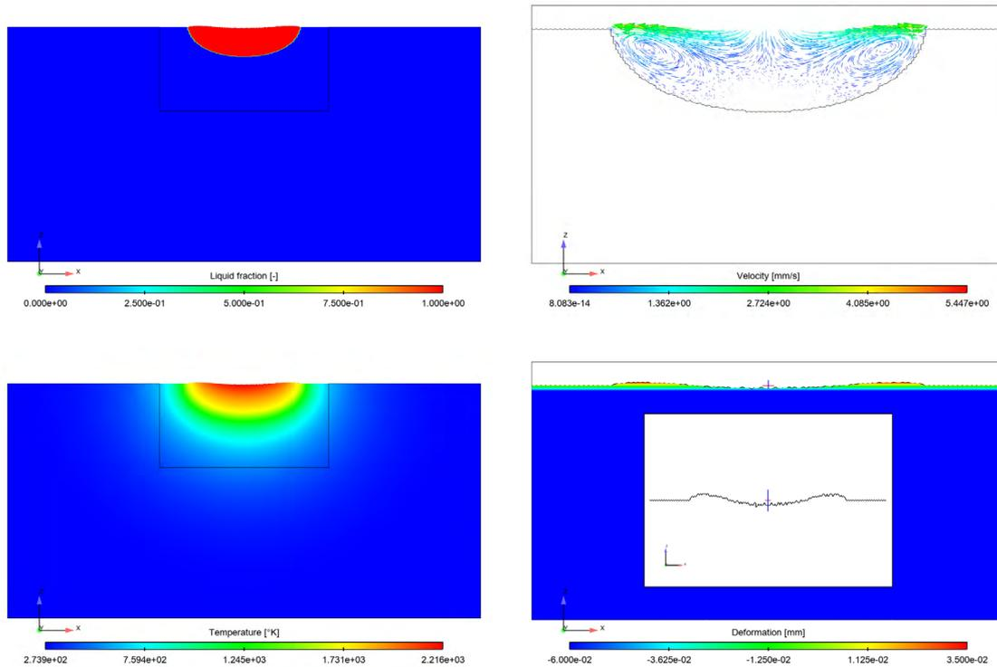
**Figure 6:** Static laser melting. Snapshots at time  $t = 1$  [s], of the numerical approximation of: the liquid fraction  $f_l$  (top left); the velocity field  $\mathbf{v}$  (top right); the temperature  $T$  (bottom left); the deformation of the free surface  $\Gamma_f$  defined by the transport of  $\varphi$  (bottom right).
