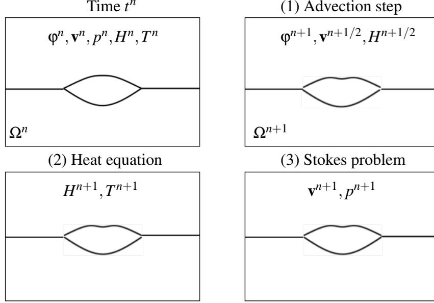
**Figure 2:** Operator splitting algorithm (from left to right, top to bottom). We solve successively (1) Three advection problems in order to obtain  $\varphi^{n+1}, \mathbf{v}^{n+1/2}, H^{n+1/2}$  and thus  $\Omega^{n+1}$ . (2) The heat diffusion equation (without convection) to determine  $H^{n+1}$  (and thus  $T^{n+1}$ ). (3) A generalized Stokes problem in order to obtain  $\mathbf{v}^{n+1}$  and  $p^{n+1}$ .
