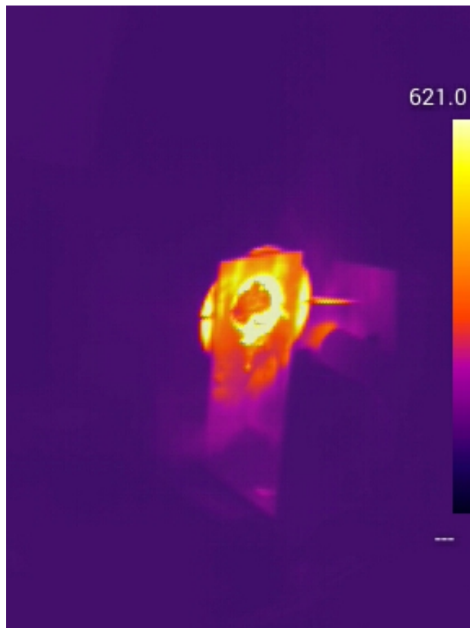
Figure C.6: Highest temperature registered by the thermographic camera, with the last specimen of configuration 4.
