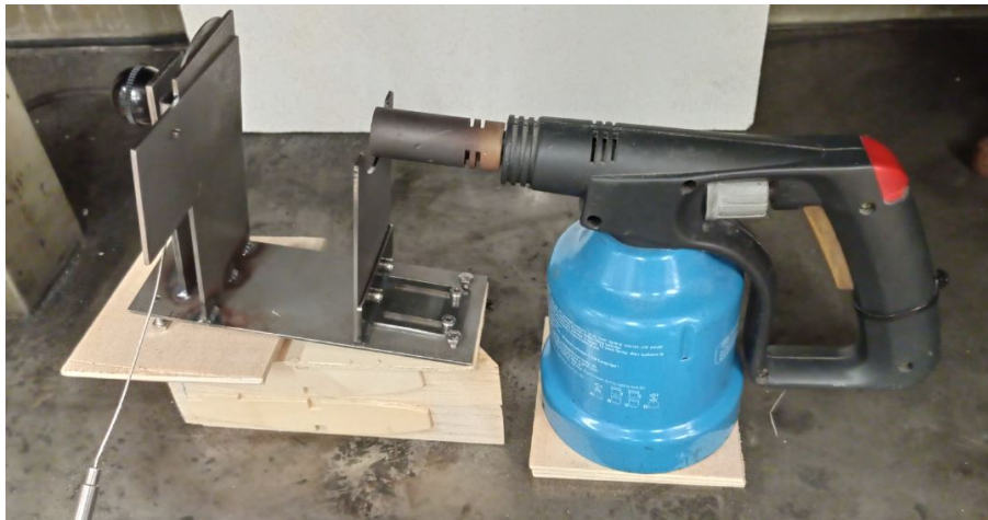
Figure 5.2: Finished experiment assembly. All of the pieces and components, including the torch and the thermocouple, can be appreciated.
