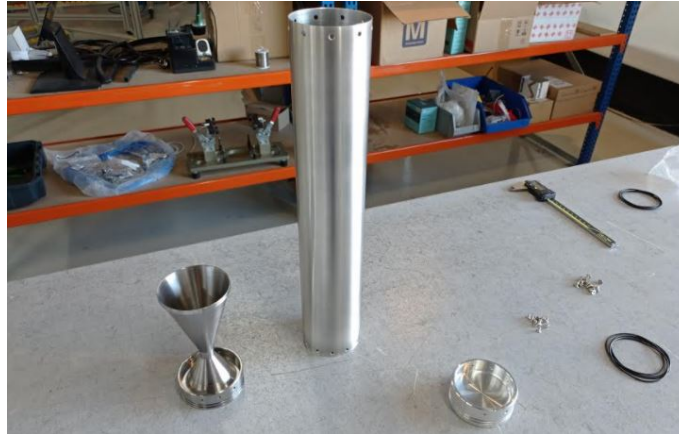
Figure 6.2: The three main engine components just before the assembly. The O-Rings and screws can be appreciated.
