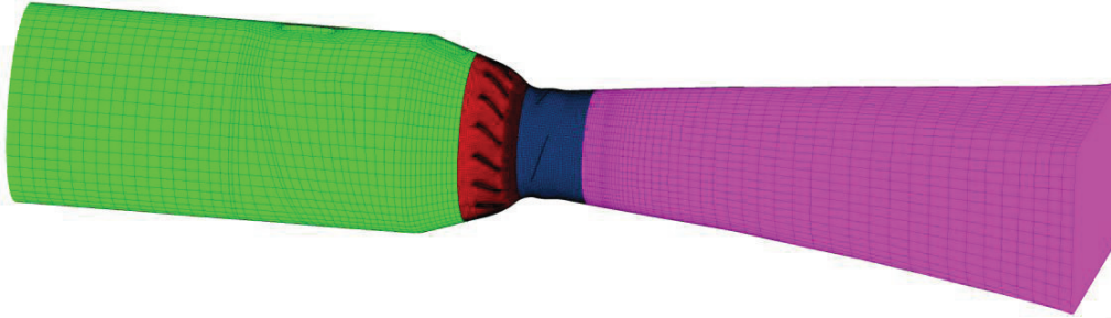
Figure 3: Mesh along the flow path
