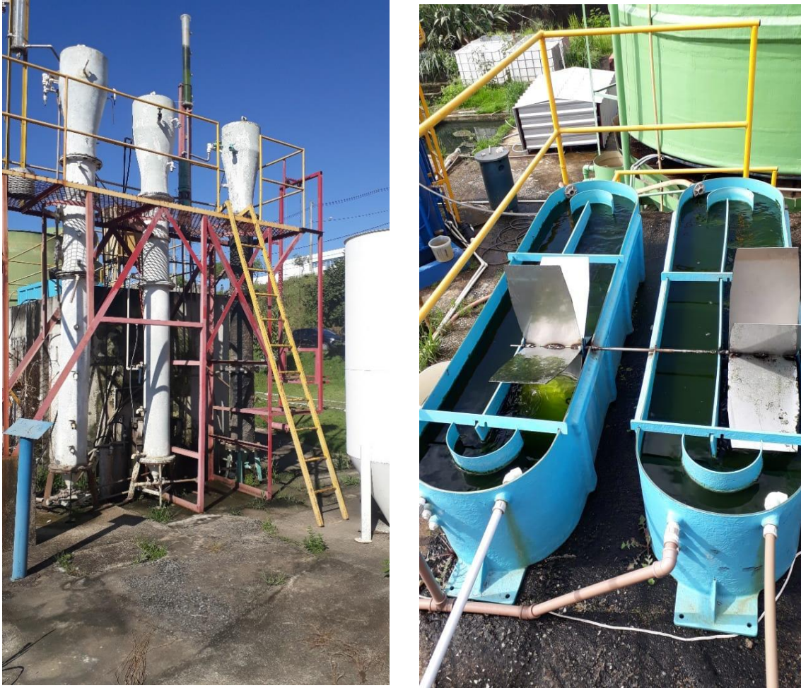
Figure 9. Photographs of the UASBs (left) and HRAPs (right) operated by the DESA (UFMG).
